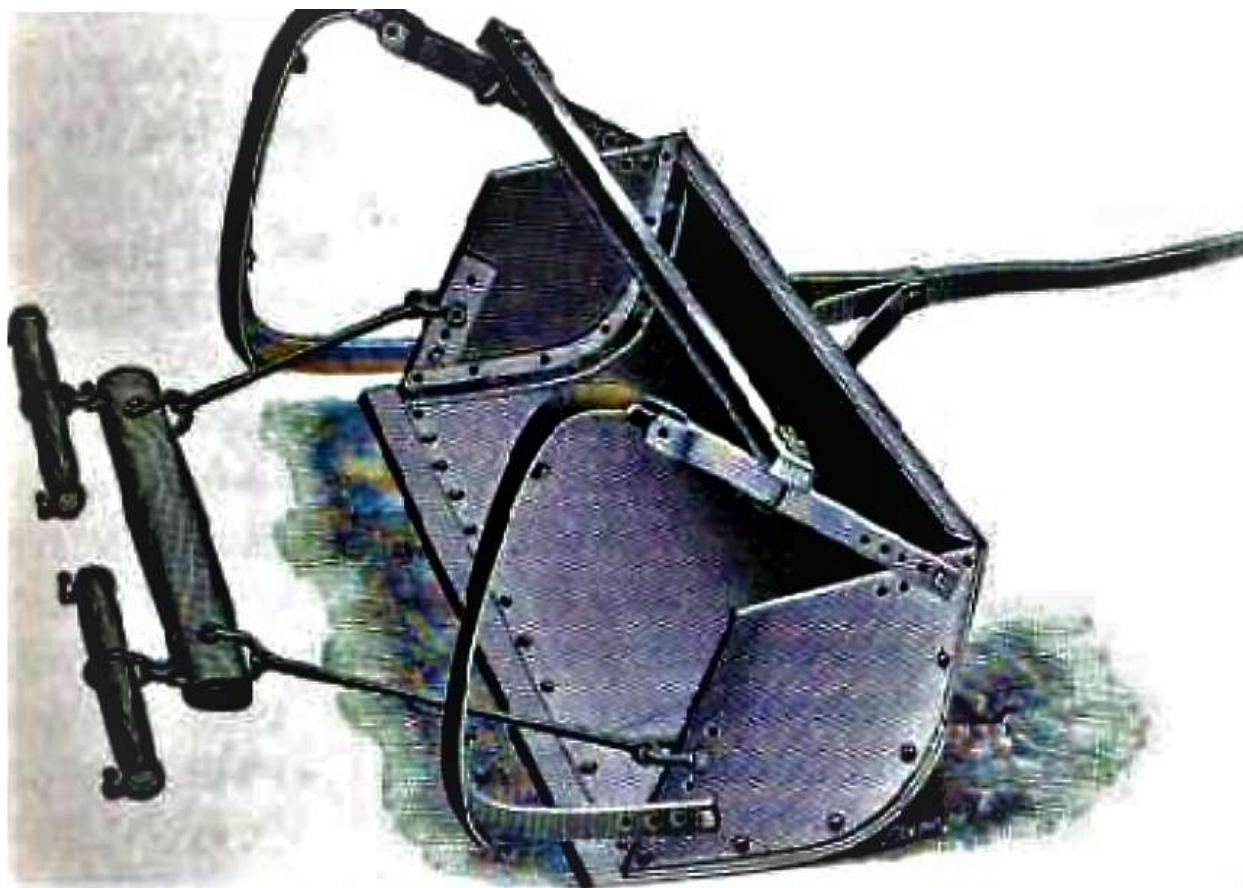
Figure 25 Fresno Scraper for harnessing to a team of two horses, by means of the attachment illustrated on the left side of this image. Note the handle on the right side of this image, by which the operator could dump the load, either all at once by raising the handle totally upright, or more gradually by raising the handle upright more gradually.
